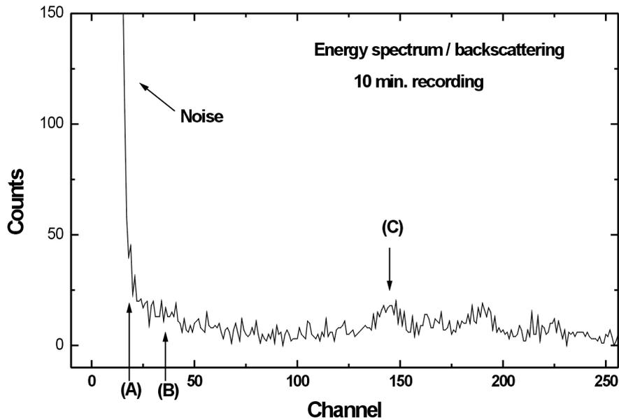
Figure 2: Energy Spectrum of a  $^{57}\text{Co}$  Mössbauer Source, taken in Backscattering Mode on the Mössbauer Calibration Target
