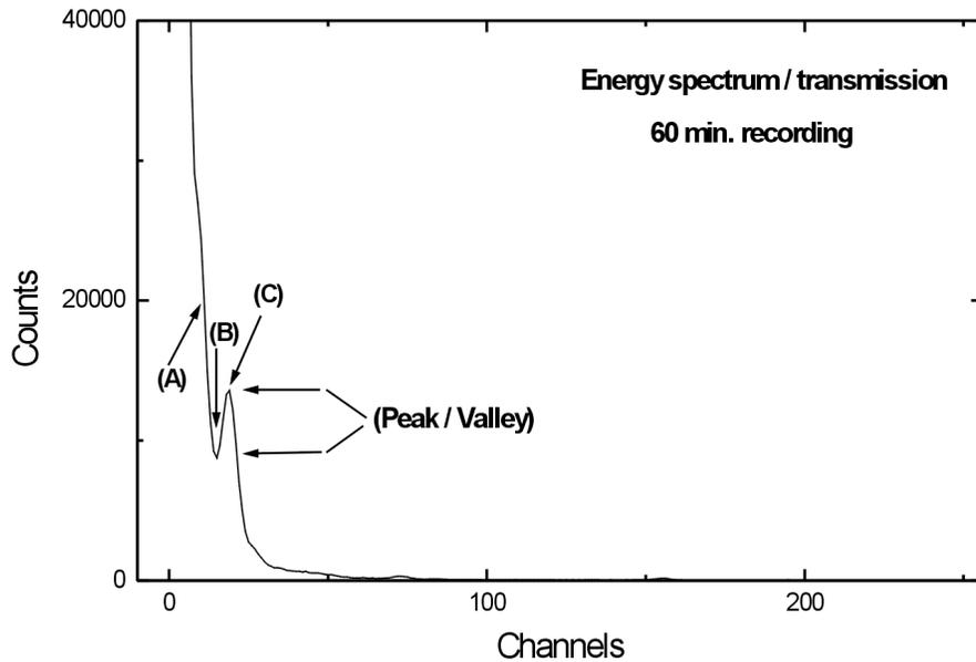
Figure 1: Energy Spectrum of a  $^{57}\text{Co}$  Mössbauer Source, taken in Transmission Mode
